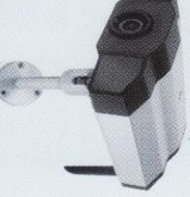
Camera Avetech KPC-138-9, Taiwan 1/3" HR color CCD image sensor Number of Pixels: 768(H) x 494(V) <NTSC> / 753(H) x 582(V) Resolution: 420 TVL Effective Range : Over 30 Meters Lens: 3.6mm / F2.0 Lens Angle: 92.6°
